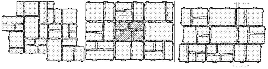
**Figure 5** Herringbone, stacked and offset laying patterns
